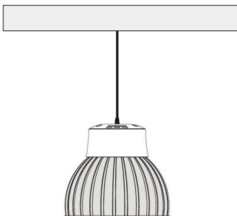
Hanging ring installation
